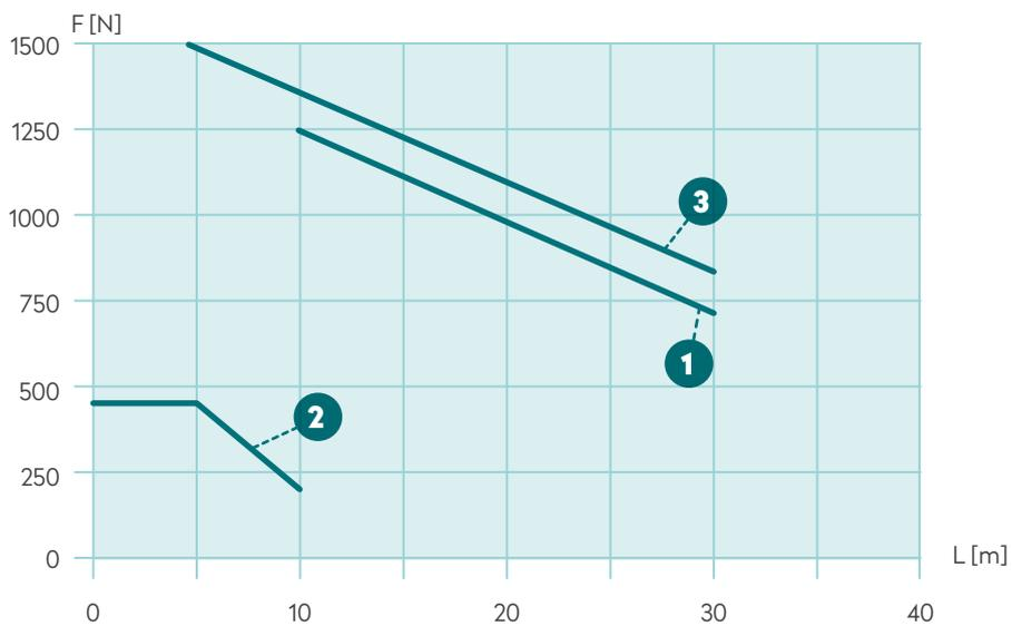
1 FS CS065/FS CS090SL (without centre drives) 2 FS CS090SL centre drives 3 FS CS200SL
