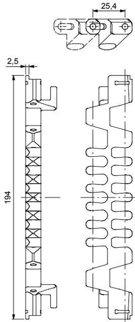
**FS CS200SL CHAIN WITH FRICTION LINING**
