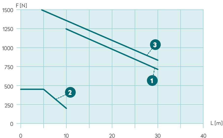
① FS CS065/FS CS090SL (without centre drives) ② FS CS090SL centre drives ③ FS CS200SL
