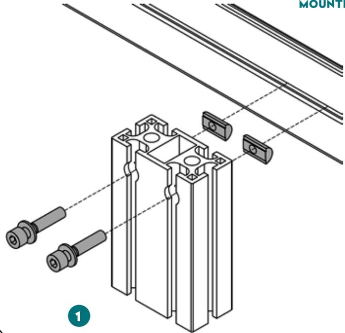
1 Socket head cap bolt, M8x40 / Washer M8
