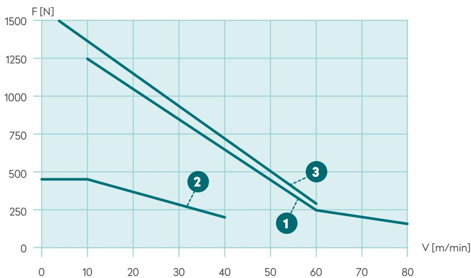
① FS CS065/FS CS090SL (without centre drives) ② FS CS090SL centre drives ③ FS CS200SL
