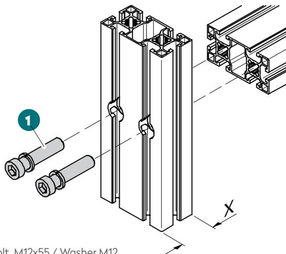
1 Socket head cap bolt, M12x55 / Washer M12
