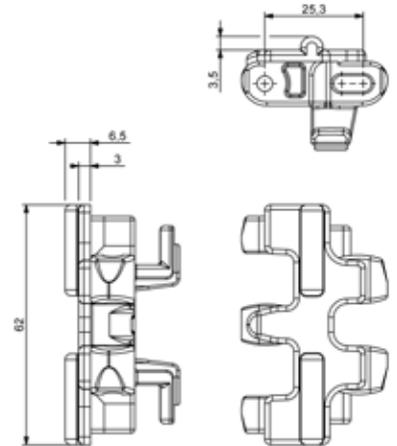
**FS CS065SL CHAIN WITH FRICTION LINING**
