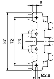
**FS CS090SL CHAIN WITH GRIPPER**
