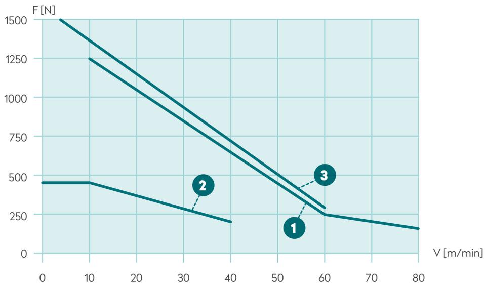
1 FS CS065/FS CS090SL (without centre drives) 2 FS CS090SL centre drives 3 FS CS200SL
